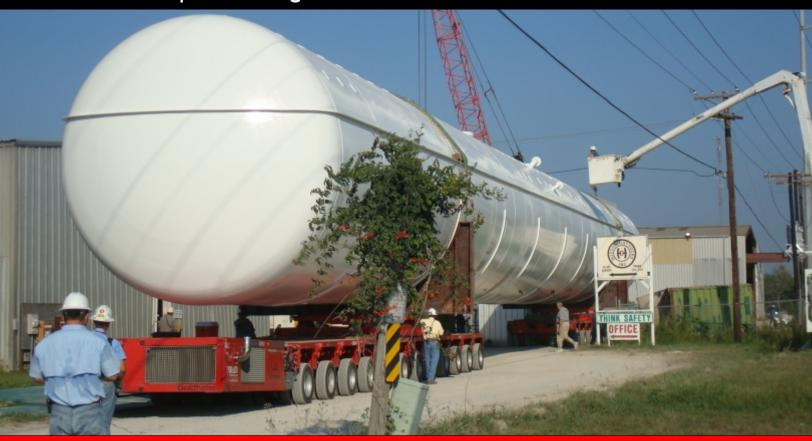
These two 200' x 17' 335 ton storage tanks were received from stands in a customer's yard and transported via city streets to an awaiting crane over a mile away. Berard provided detailed descriptions of transport path throughout the move, including detailed drawings showing exactly where matting would be needed, or where objects would need to be removed. Despite sweltering temperatures nearing 100 degrees, the people, equipment, and plan worked flawlessly in time and under budget.
